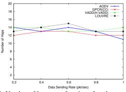
Fig. 10: Number of hops as a function of packet sending rate - TAPAS/Cologne
