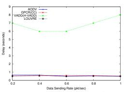
Fig. 9: Packet delivery delay as a function of packet sending rate - TAPAS/Cologne
