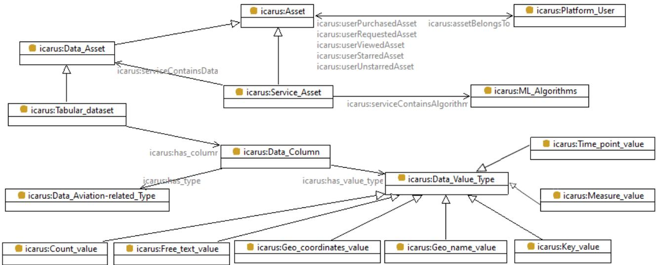
Figure 4: Relations of the main classes and sub-classes of the top ontology
