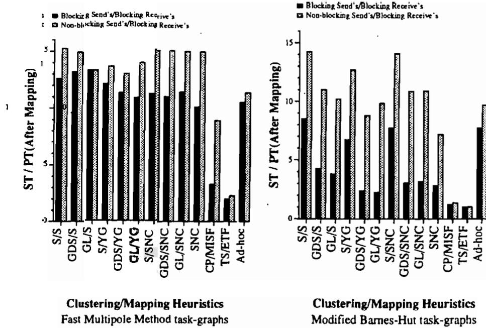
Figure 8 Speedups for different clustering-mapping strategies (16 processors).
