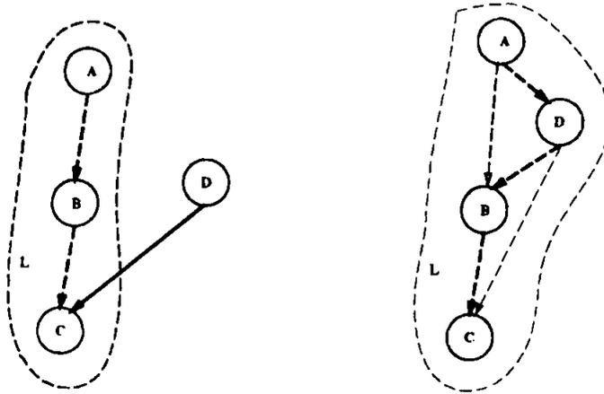
Figure 3 Scheduling edges. The bold arrows denote the sequential paths of execution in the clusters.
