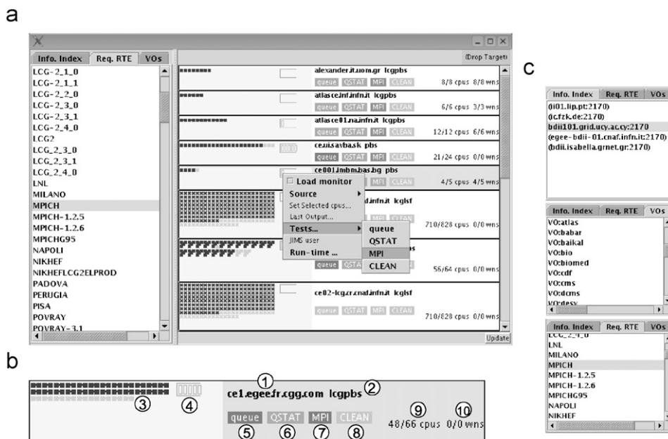
Fig. 10. (a) Resource browser, showing the state of resources from the EGEE test-bed that “advertise” support for MPI (MPICH run-time environment); (b) the resource renderer; (c) *top*: information index sources selection. *Middle*: querying for specific Virtual Organizations. *Bottom*: specifying run-time environment support.
