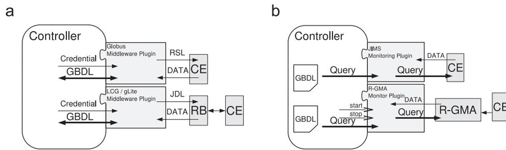
Fig. 7. Left: Middleware plugin functionality. Right: Monitor plugin functionality.
