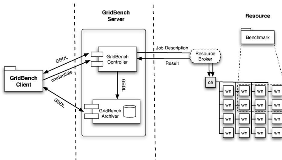
Fig. 3. GridBench component communication.
