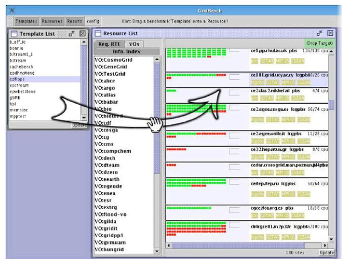
Fig. 8. The list on the left is a list of tests/benchmarks that are integrated into GridBench. The list on the right shows the currently available resources and their status in terms of busy/free CPUs.
